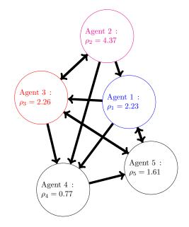
Fig. 3. Graph structure under consideration. An arrow from m to m implies that agent m is influenced by agent t and  $A_{n,m} = 1$ , otherwise  $A_{n,m} = 0$ . We compute  $\rho_n$  using (12) for T = 1.
