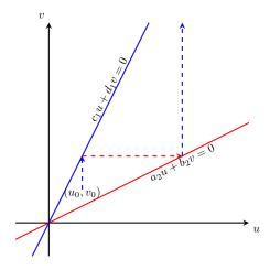
Fig. 2. The slow manifold associated with (19) and (20) when  $\frac{|c_1b_2|}{|d_1a_2|} > 1$ . The dashed lines represent the asymptotic behavior of the overall system with initial state  $(u_0,v_0)$  when  $\varepsilon \to 0$  and no dwell-time (or  $\mathcal{O}(\varepsilon)$  dwell-time) is imposed. It is illustrated that in this case a dwell-time of order  $\frac{\ln(\gamma_{11})}{\lambda_s} + \mathcal{O}(\varepsilon)$  has to be imposed in order to guarantee the system's stability.
