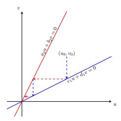
Fig. 1. The slow manifold associated with (19) and (20) when  $\frac{|c_1b_2|}{|d_1a_2|} < 1$ . The dashed lines represent the asymptotic behavior of the overall system with initial state  $(u_0,v_0)$  when  $\varepsilon \to 0$  and no dwell-time (or  $\mathcal{O}(\varepsilon)$  dwell-time) is imposed. It can be seen that system (19)-(20) is asymptotically stable for any switching rule.
