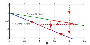
Fig. 6. First part of the state's trajectory in (u,v)-plane for (19)-(20) with  ${\bf A}_1, {\bf A}_2$  defined by (23) and  $t_{k+1}-t_k=\tau=0.406~sec$
