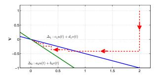
Fig. 4. State's trajectory in (u,v)- plane for (19)-(20) with  $\mathbf{A}_1,\mathbf{A}_2$  defined by (22) and  $t_{k+1}-t_k=\tau=6.16\cdot 10^{-4}=O(\varepsilon)$  sec. Note that first switches take place before the trajectory reaches the slow manifolds. Unlike Figures 1 and 2 here we see the trajectory of the system for a fixed  $\varepsilon$  and not the limiting behavior when  $\varepsilon\to 0$ .
