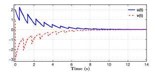
Fig. 5. State's trajectory for (19)-(20) with  ${\bf A}_1, {\bf A}_2$  defined by (23) and  $t_{k+1}-t_k=\tau=0.406~sec$
