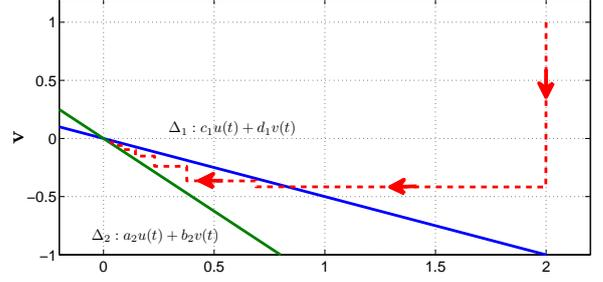
Fig. 4. State's trajectory in  $(u, v)$ - plane for (19)-(20) with  $\mathbf{A}_1, \mathbf{A}_2$  defined by (22) and  $t_{k+1} - t_k = \tau = 6.16 \cdot 10^{-4} = \mathcal{O}(\varepsilon)$  sec. Note that first switches take place before the trajectory reaches the slow manifolds. Unlike Figures 1 and 2 here we see the trajectory of the system for a fixed  $\varepsilon$  and not the limiting behavior when  $\varepsilon \rightarrow 0$ .
