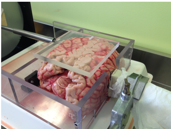
Figure 11: Ex vivo human brain with probe and vibrating plate
