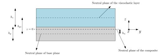
Figure 3: Slice of the 3d plate. The shape  $\mathcal{O}$  belongs to the xy-plane, being x the outward axis in the figure.
