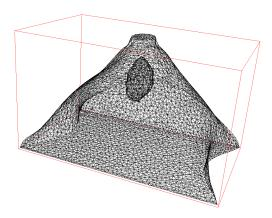
Figure 5: The optimized shape possesses a small inner cavity. If the hole is filled with the viscoelastic material, the value of  $\eta$  remains almost constant (actually it slightly diminishes) so the value of the composite objective function (58) increases. The authors verified that the inner cavity is not present when the whole working domain  $\mathcal{O}$  is used as initial shape in the optimization process.
