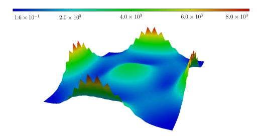
Figure 9: In-plane extensional strain energy density  $({\rm J/m^2}).$
