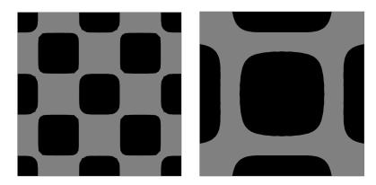
Figure 7: Initial and optimized shapes of the composite plate. The aluminum phase is shown in gray and the (superposed) viscoelastic one in black.
