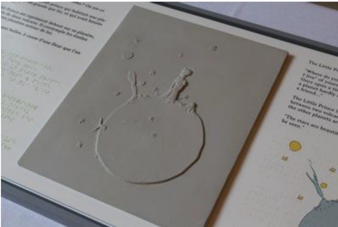
Fig. 1. Tactile image produced using the thermoforming illustration technique. "The Little Prince" of Antoine de Saint-Exupéry. Illustration from [31]
