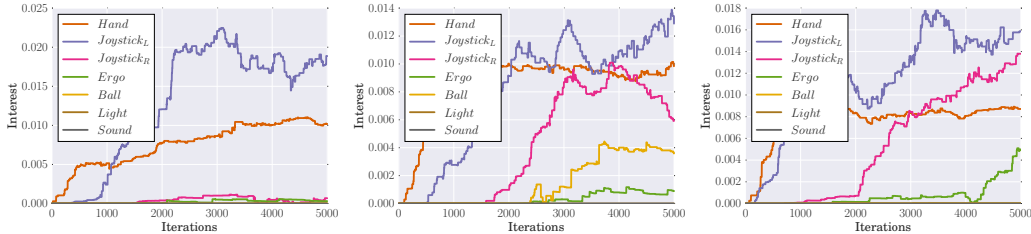
Figure 5: Intrinsic Rewards in condition AMB. Each graph shows the learning progress estimated by one agent of condition AMB in each of the problem spaces during the 5000 iterations. The learning progress heuristic leads to a sequence of exploration focus from easier to more complex problems.
