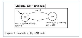
Automaton consists of states, one of them being the initial state, and transitions between them. States are associated to equations that give specific values to the output flows of the automaton node. The value of an output flow must be defined at each instant. Transitions are associated to boolean expressions related to one or several input flows of the automaton node.
