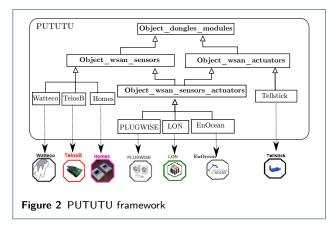
hides their heterogeneity. PUTUTU consists of several LINC objects. As shown in Figure 2, these objects encapsulate different technologies (e.g., TelosB, LON, Tellstick) and inherit from four generic objects:
