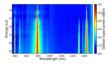
Fig. 6. Energy map from 7  $\mu$ J (49 MW/cm<sup>2</sup>) to 37  $\mu$ J (261 MW/cm<sup>2</sup>).
