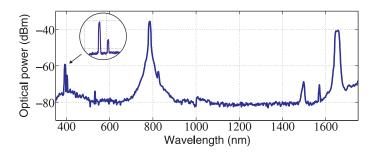
Fig. 3. Full spectrum measured at a peak power of 40 kW with a resolution of 5 nm from 350 nm to 1750 nm at 110  $^{\circ}$ C. The inset is a zoom-in spectrum around 400 nm.
