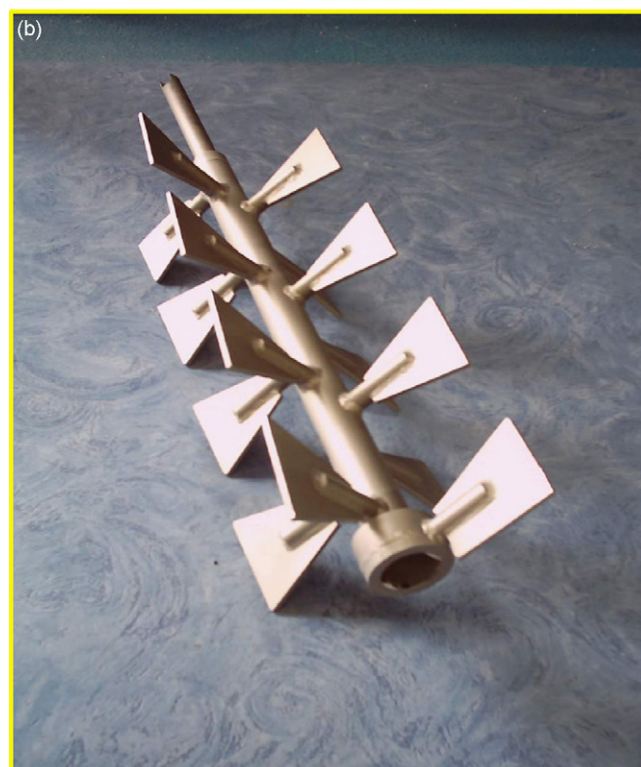
Fig. 1. Pilot plant equipment (a) used showing the loss-in-weight feeders, and stirring device (b).
