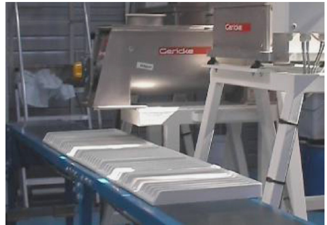
Fig. 2. Photograph of the outlet of the mixer showing the sampling set-up.
