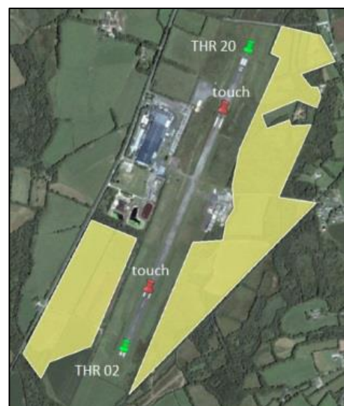
Figure 4: Superimposing the footprint of the ground-based PV plant (yellow) with the satellite image; thresholds (THR) and touchdowns are highlighted.
