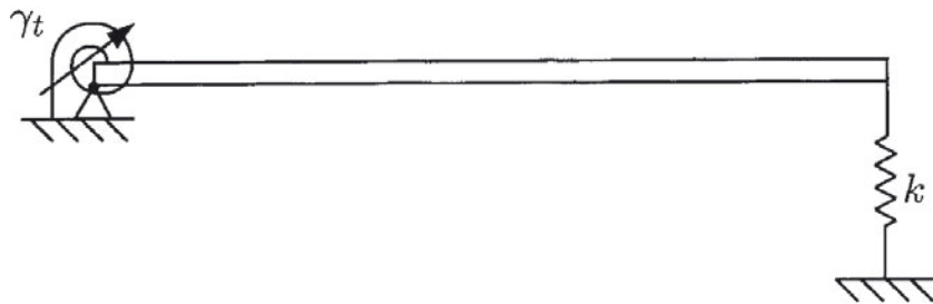
Figure 7. Schematic of finite element model: 200 beam elements were used to construct a beam with: L = 1 m, \rho = 7860 kg/m 3 , E = 2 \times 10^{11} N/m 2 , I = 5 \times 10^{-8} m 4 . The parameters k and \gamma_t vary by case.
