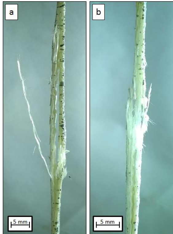
Figure 16 – Side view of LD samples with short fatigue life: \sigma_{max} = 194 \text{ MPa} (a) and \sigma_{max} = 111 \text{ MPa} (b)
