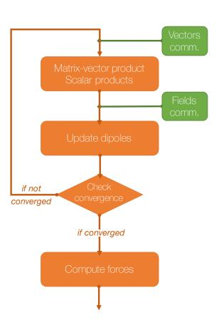
Figure 4: schematic representation of an iteration of a polarization solver
