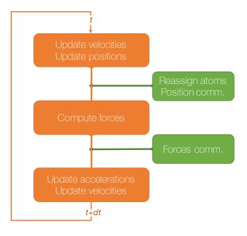
Figure 3: schematic representation of a velocity verlet step
