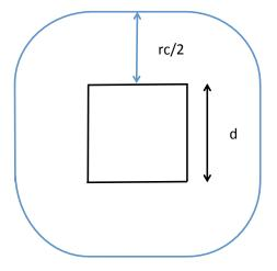
Figure 2: illustration of the midpoint rule in 2D: the square of edge d represents a subdomain assigned to a process and the blue line delimits the area that has to be imported by the latter
