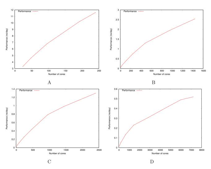
Figure 6: performance gain for the [dmim+][cl-] ionic liquid system (A) and the Puddle (B), Pond (C) and Lake (D) water boxes
