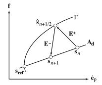
Fig. 4 An iteration of the LATIN method
