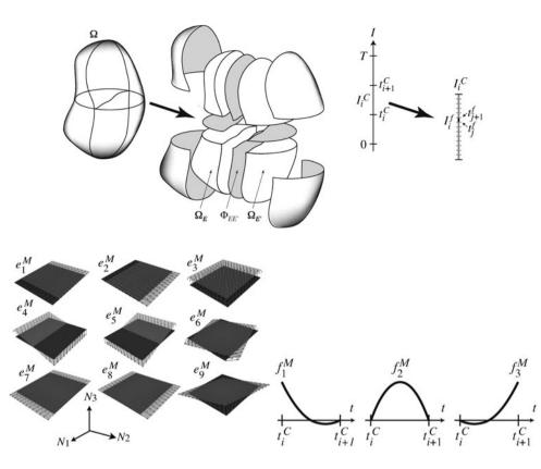
**Fig. 8** The linear macro basis in space for a square interface  $\Phi_{EE'}$  in the 3D case, and the quadratic macro basis in time over  $I_i^C$
