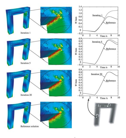
problem in both the space domain and the time domain. After a few iterations, the solution becomes even more accurate and the stress and displacement discrepancies tend toward zero. After 20 iterations, the difference between the approximate solution and the reference solution is no longer visible.
