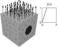
Fig. 13 Description of a micro problem corresponding to a Type-II substructure and its loading
