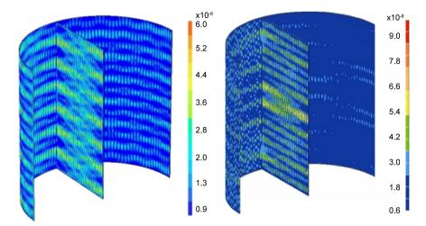
Fig. 8. Comparison of the displacements (in m) obtained using the VTCR (left with 264 DOFs) and the FEM program MSC Nastran (right with about 1,200,000 DOFs) for the problem of Section 4.3 illustrated in Fig. 7.
