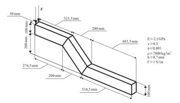
Fig. 3. Definition of the example problem of Section 3.3: an assembly of 12 plates subjected to a shear force F distributed linearly along an edge.
