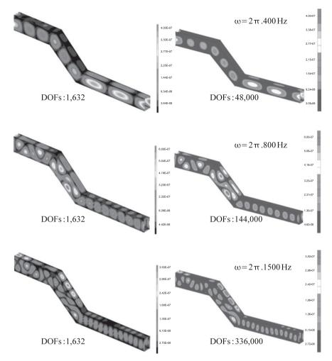
**Fig. 4.** Comparison of the normal displacements (in m) obtained using the VTCR (left) and the FEM program MSC Nastran (right) for the problem of Fig. 3. The numbers of DOFs used and the circular frequencies considered are given next to each plot.
