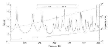
**Fig. 13.** Comparison of the FRFs given by the FEM and the VTCR for the problem of Section 5.3 illustrated in Fig. 11. The corresponding numbers of DOFs are indicated on the vertical scale on the right. For the FEM, 14 elements per wavelength were used. For the VTCR, the number of shape functions was chosen so that the relative error compared to the FEM would be less than  $10^{-3}$  for each frequency.
