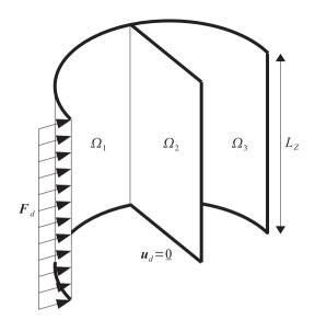
Fig. 7. Definition of the example problem of Section 4.3: an assembly of two cylindrical shells and one plate.
