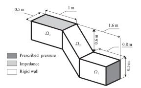
Fig. 11. Problem definition for the Z-shaped cavity filled with air of Section 5.3.
