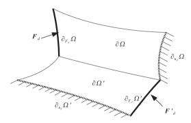
Fig. 5. Problem definition of the 3D assembly of two shells.
