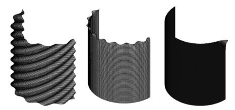
**Fig. 6.** Interior, edge and corner waves which satisfy (16) for a homogeneous cylinder. The nature of the wave depends on the real and imaginary parts of the coordinates of **k** in function e<sup>*i*k x</sup>.
