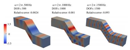
Fig. 12. The real part of the VTCR pressure for the problem of Section 5.3 illustrated in Fig. 11. The circular frequency considered, the number of DOFs and the relative error are indicated in each case.
