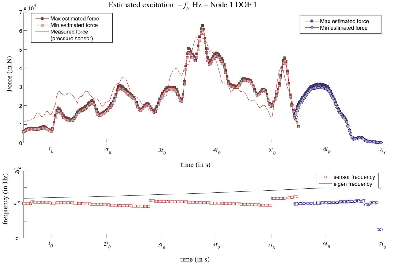
Fig. 7. Estimate of excitation corresponding to the 1<sup>st</sup> acoustic mode.
