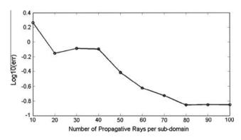
**Fig. 12.** Error of the complex frame structure example presented in Section 4.2. The definition of the error is given in Eq. (60). Convergence is achieved around 80 propagative rays per subdomain (1224 total DoFs). The remaining error (around 10%) stays stable afterwards and it is due small differences in theories. The reference solution is computed by ABAQUS® using 372084 DoFs.
