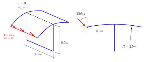
Fig. 10. Boundary conditions and geometric dimensions of the complex frame structure described in Section 4.2.
