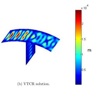
Fig. 11. Magnitude of the displacement of the vibrational problem of Section 4.2.
