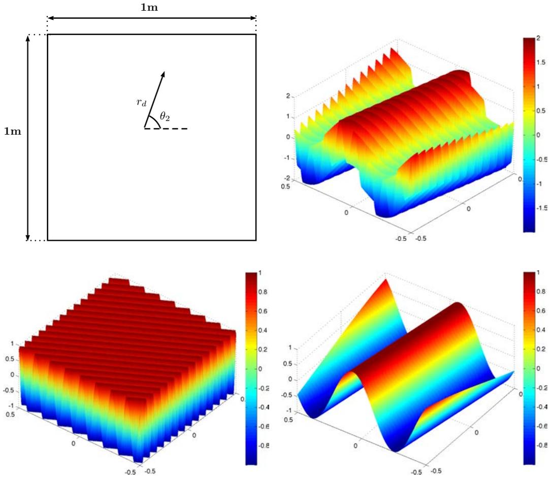
Fig. 5. Example considered in Sec. 3.2. Up left: Definition of the computational domain. Up right: Exact solution  $u_{\text{exact}}$ . Down left: Representation of the fast varying scale result simulated by VTCR part  $u_{\text{VTCR}}$ . Down right: Representation of the slow varying scale result simulated by FEM part  $u_{\text{FEM}}$ .
