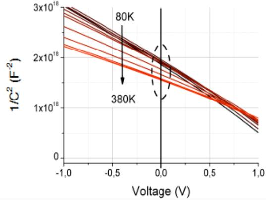
Fig. 2 — Low voltage  $1/C^2$  measurement on device B.
