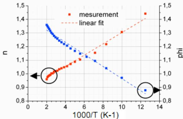
Fig. 3 — Dependence of ideality factor and barrier height versus temperature.
