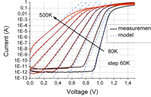
Fig. 5 — Forward bias measurement vs. new fitting technique of device C.
