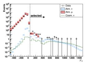
Figure 12: Left: RDF parameter for data, cosmic neutrinos and atmospheric background. This figure corresponds to the event distributions after all the cuts prior to the RDF listed in Table 2. Right: muon likelihood ratio parameter for data, cosmic neutrinos and atmospheric background. This figure corresponds to the event distributions after the RDF and all previous cuts listed in Table 2. In both figures the dashed vertical line indicates the cut value.
