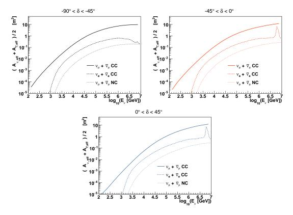
Figure 1: Effective area for  $\nu_{\mu}+\bar{\nu}_{\mu}$  CC events after the track selection cuts (solid line) and for  $\nu_{e}+\bar{\nu}_{e}$  CC and  $\nu_{\mu}+\bar{\nu}_{\mu}$  NC events after the shower selection cuts (dashed lines) considering three declination ranges.
