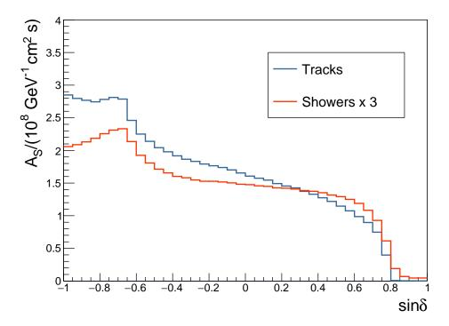
Figure 5: The acceptance as a function of the source declination for an  $E^{-2}$  energy spectrum with a flux normalization factor of  $\Phi_0 = 10^{-8} \,\text{GeV} \,\text{cm}^{-2} \,\text{s}^{-1}$  for the track (blue) and shower (red) samples. For better visibility, the acceptance for showers is scaled up by a factor 3.
