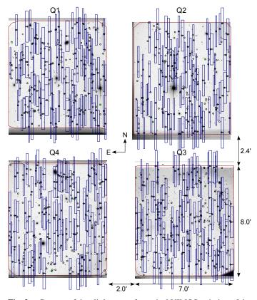
**Fig. 3.** Cartoon of the slit lay-out of a typical VIMOS pointing of the VIPERS survey (W1P082 in this case), superimposed on the actual DSS finding chart. The open circles with the tiny horizontal slits mark the target objects. The vertical rectangles define the area where the resulting spectrum will fall, once the dispersing element (grism) is inserted.
