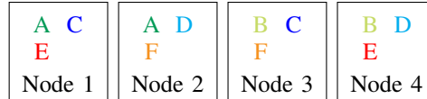
Figure 2. Example of uniform data distribution with 4 nodes and a replication factor of 2, every two nodes share 1/3 of their data (A to F).
