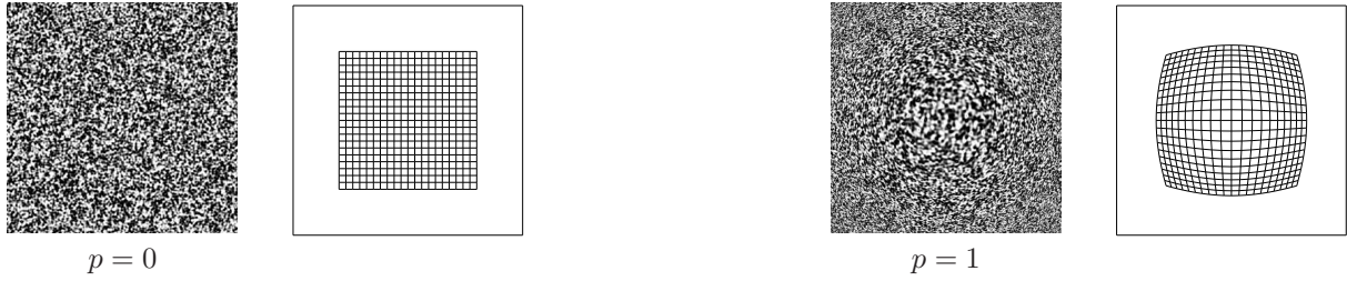
Figure 7. Punch function. We show two results obtained with different values of the parameter p of the punch function; r = 0.8 . The meshes give a better idea of how the original pattern is deformed by tracking the displacements of the points on a regular grid.
