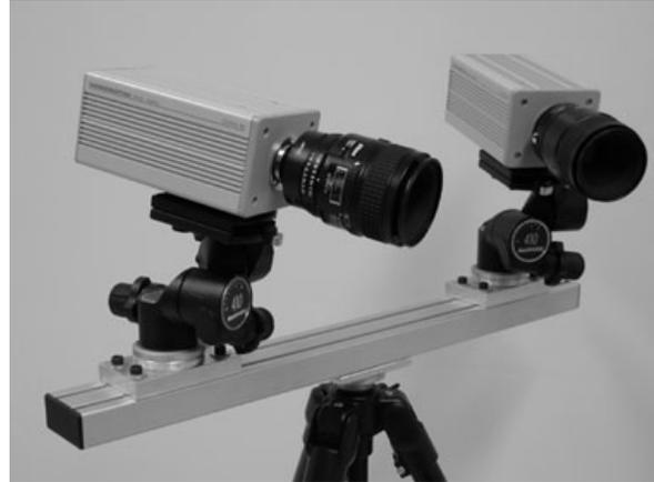
Figure 2: The stereo-rig used in our laboratory
