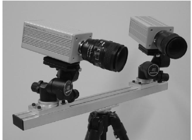
Fig. 2. The stereo rig used in our lab.
