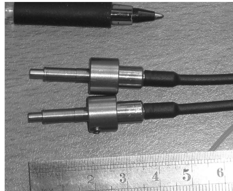
Figure 4. FBG contact pressure and temperature sensor.
