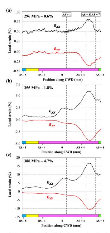
**Fig. 10.** Mean  $\epsilon_{XX}$  and  $\epsilon_{YY}$  values along CWD for various stress/strain conditions. a) 296 MPa-0.6%, b) 355 MPa-1.8% and c) 388 MPa-4.7% showing local strain concentration areas.
