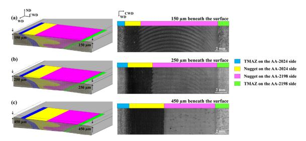
**Fig. 5.** Macrostructure of the dissimilar joint at various CWD-WD sections showing the occurrence and the disappearance of banded macrostructures in the shoulder-affected region: (a) at 150 μm beneath the top surface, (b) at 250 μm beneath the top surface, (c) at 450 μm beneath the top surface.
