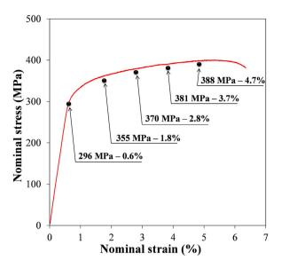
**Fig. 4.** Macroscopic stress-strain behavior corresponding to the shoulder-affected region of the joint and the macroscopic strains measured by crosshead displacements at the various holding stress for which OHR-DIC measurements were made (black dots).
