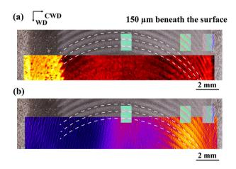
**Fig. 12.** Correlation between banded macrostructure, local mechanical properties and crystallographic texture. The ⟨110⟩ fiber aligned with the metal flow direction (green area on the EBSD scan) correspond to HDB and LHB. (a) Emphasis on HHB/LHB pattern. (b) Emphasis on HDB/LDB pattern.
