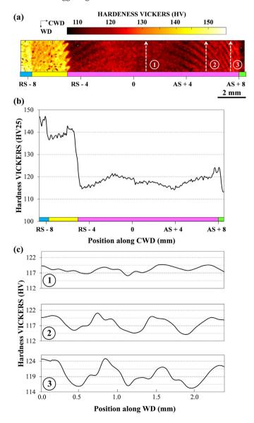
**Fig. 8.** (a) Hardness map across the WD-CWD plane located 150  $\mu$ m beneath the top surface. (b) Mean hardness values along CWD (The mean hardness value is calculated by integrating the entire measurements for a given coordinate). (c) Mean hardness values along WD for three locations in the AA-2198 nugget region corresponding to the dashed white lines in Fig. 8.a obtained at AS + 1 mm, AS + 5 mm and AS + 7 mm.
