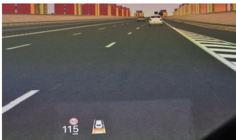
Figure 5. Classical HUD with warning icon in MD
