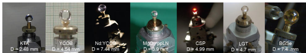
Fig. 4. Examples of polished spheres mounted on goniometer heads for optical measurements.
