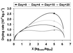
Fig. 17. Influence of the storage during on the drying kinetic behavior of wastewater sludge [43].
