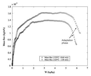
Fig. 6. Experimental results of wastewater sludge convective drying [35].
