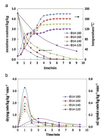
**Fig. 23.** Influence of the oil temperature on the sludge drying behavior during frying [55], (a) Variation of the product moisture content and its temperature, (b) drying rate.
