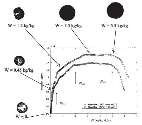
Fig. 11. Shrinkage and cracks formation during convective drying [36].
