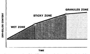
Fig. 18. Presentation of the different phases during conductive drying [8].
