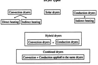
Fig. 1. Types of dryers used for sludge wastewater drying [2].
