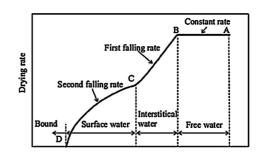
Fig. 5. Typical wastewater sludge drying curve [1].
