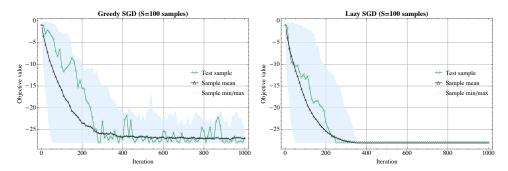
Figure 5. Convergence of the lazy and greedy variants of SGD in a quadratic minimization problem of the form (7.1) with d = 100. The lightly shaded area traces the best and worst realizations of the algorithm over S = 100 sample runs; the corresponding sample mean is drawn as a solid black line. In the dedicated runtime (n = 1000 iterations), the greedy variant still hasn't converged; by contrast, even the worst realization of lazy SGD has converged within approximately 300 iterations.
