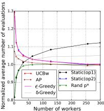
Figure 2: Normalized average number of evaluations as a function of batch size using 128 workers (top), and as a function of the number of workers using a batch size 128 (bottom). The values are normalized by the average number of evaluations of the heterogeneous random strategy with p=0.5. The lower the better.
