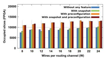
**Fig. 7.** Occupied resources in terms of total used slices for the synthesis of a 10x10 CLBs overlay on Xilinx Artix-7 varying *W*.
