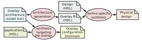
Fig. 3. Two flows: overlay synthesis on the FPGA, and application synthesis on the overlay.
