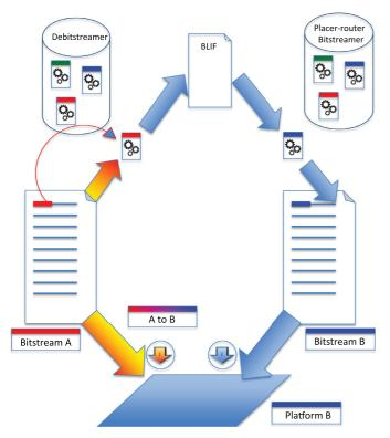
Fig. 4. Ensuring backward bitstream compatibility.
