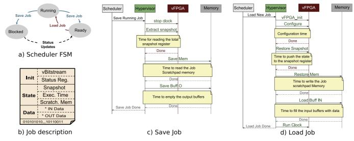
Fig. 11. The entire software layer and functions: a) remind of the classical scheduler FSM, b) the proposed Job structure, c) the sequence diagram of the save job action, and d) the one for the load job action.
