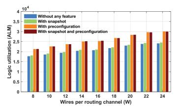
**Fig. 8.** Occupied resources in terms of Adaptive Logic Module (ALM) for the synthesis of a 10x10 CLBs overlay on Altera Cyclone-V varying W.
