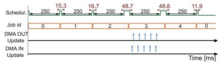
Fig. 15. Execution of the jobs for an ETRR scheduling with Q = 250 ms.
