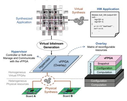
Fig. 1. Overview of the proposed FPGA virtualization approach.
