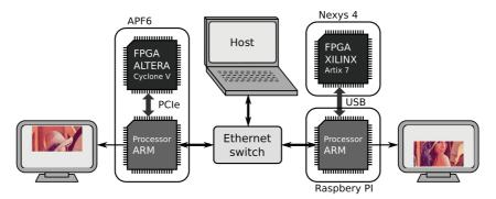
Fig. 13. Experimental setup of the DASIP demonstration.
