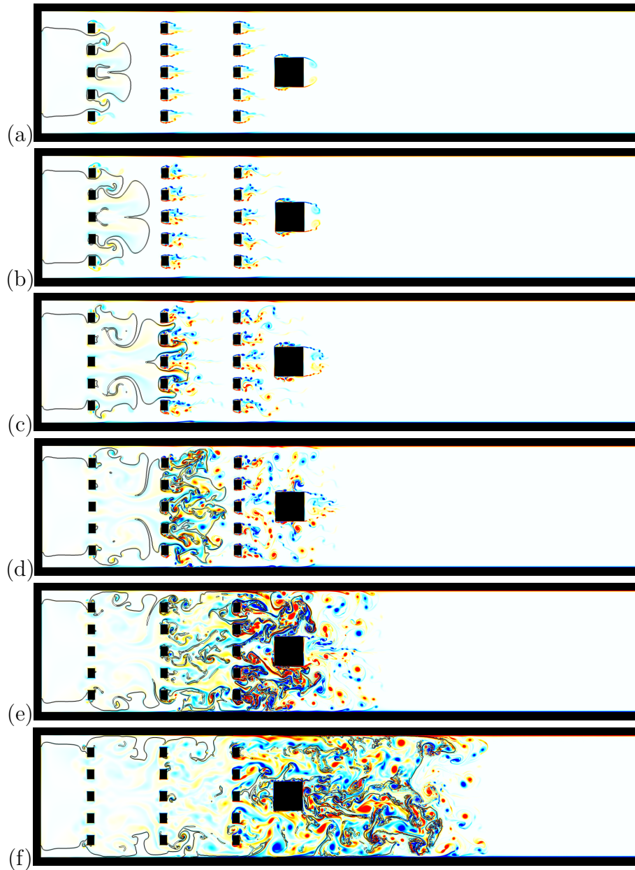
Figure 4: Simulation 2D-DNS1. Snapshots of the vorticity field with isocontours of the progress variable ( c = 0.2 and c = 0.8 ) that indicates the flame front for: (a) t = 4 ms, (b) t = 4.5 ms, (c) t = 5 ms, (d) t = 5.5 ms, (e) t = 6 ms and , (f) t = 6.5 ms. The red color corresponds to \Omega_z = 5 \times 10^4 s -1 , while blue corresponds to \Omega_z = -5 \times 10^4 s -1 .
