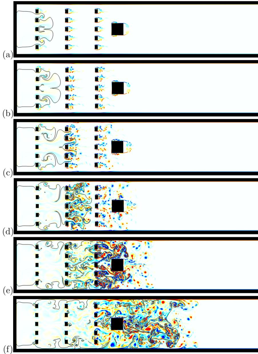
Figure 4: Simulation 2D-DNS1. Snapshots of the vorticity field with isocontours of the progress variable ( $c = 0.2$  and  $c = 0.8$ ) that indicates the flame front for: (a)  $t = 4$  ms, (b)  $t = 4.5$  ms, (c)  $t = 5$  ms, (d)  $t = 5.5$  ms, (e)  $t = 6$  ms and , (f)  $t = 6.5$  ms. The red color corresponds to  $\Omega_z = 5 \times 10^4$  s<sup>-1</sup>, while blue corresponds to  $\Omega_z = -5 \times 10^4$  s<sup>-1</sup>.
