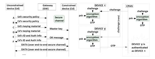
**Fig. 1.** Association and secure channel establishment solution
