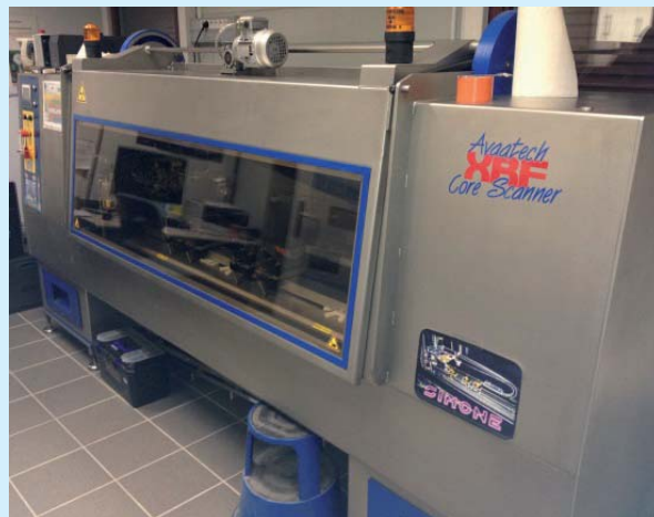
Avaatech XRF core scanner.
