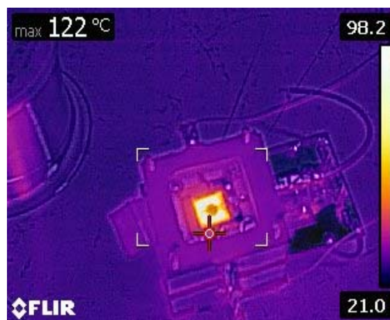
Fig. 4. FLIR image of the detection cell with a 35 mA heating current through the 30 nm thick aluminum meander.
