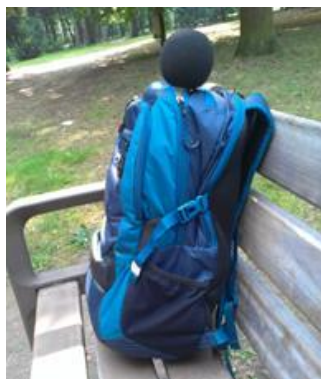
Figure 2 Backpacked sound measurement station.
