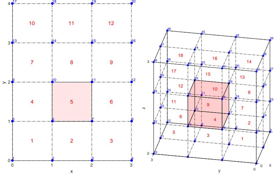
Figure 3: In blue, vertices of cartesian Grid in  $\mathbb{R}^d$  with their indices in  $\mathbf{q}$  array,  $d = 2$  and  $N_1 = 3, N_2 = 4$  (left),  $d = 3$  and  $(N_1, N_2, N_3) = (2, 3, 3)$  (right). The red numbers are the indices of unit hypercubes in the array  $\mathbf{me}$ .
