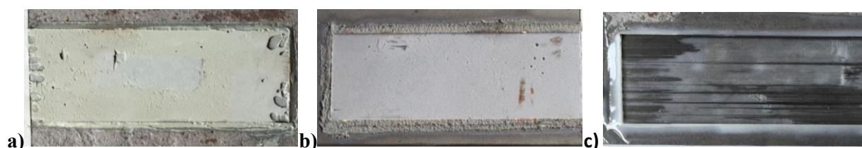
Figure 1: Photos of the obtained failure modes (reinforcement processes A, B and C)
