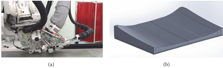
FIGURE 4: (a) An example of a fiber placement robot and (b) of a piece for the automotive industry.
