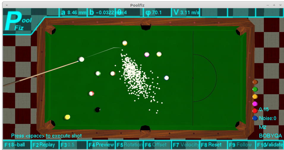
Figure 11: In this shot to the upper side pocket, we are able to see a number of possible positions at which the cue ball will end after being simulated 500 times with random gaussian noise added to the parameters.
