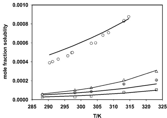
**Figure 5.** Solubility of benzoic, ferulic, caffeic, and *trans*-cinnamic acids in water. Symbols represent experimental data: (○) benzoic acid, (△) caffeic acid, (□) *trans*-cinnamic acid, and (⊕) ferulic acid. Modeling results: benzoic acid,  $k_{ij} = -0.04$ ; ferulic acid,  $k_{ij} = -0.13$ ; caffeic acid,  $k_{ij} = -0.10$ ; and *trans*-cinnamic acid,  $k_{ij} = -0.05$ .
