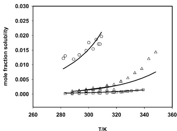
**Figure 4.** Solubility of phenol, gallic acid, and salicylic acid in water. Symbols represent experimental data: (○) phenol, (△) gallic acid, and (□) salicylic acid. Modeling results: phenol,  $k_{ij} = -0.02$ ; gallic acid,  $k_{ij} = -0.13$ ; and salicylic acid,  $k_{ij} = -0.06$ .
