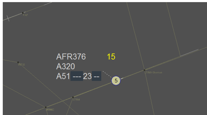
Fig. 4. Advisory countdown (yellow) shown at the controller radar display
