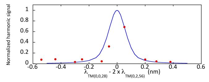
**Figure 4.** Experimental (dots) and calculated (full line) harmonic signal as a function of the detuning between harmonic and pump. The vertical scale for the experimental data has been adjusted so that the measurement for the 7616 nm diameter disk corresponds to the modeling. The experimental points correspond to data partially shown on Fig. 3.
