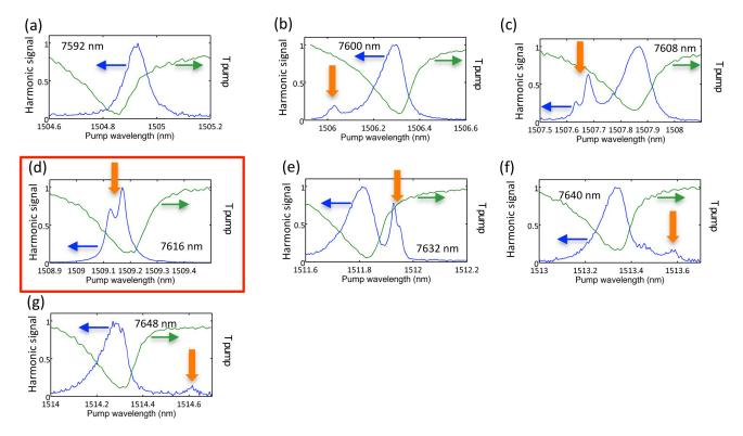
**Figure 3.** (a-g) Spectral dependence of the second harmonic signal as a function of the pump wavelength for different disk diameters indicated in the graphs in nm. The green curve corresponds to the pump transmission. The blue curve corresponds to the normalized harmonic signal. The resonant enhancement at the harmonic frequency is indicated by arrows. The red square highlights the structure where phase-matched harmonic generation is obtained.
