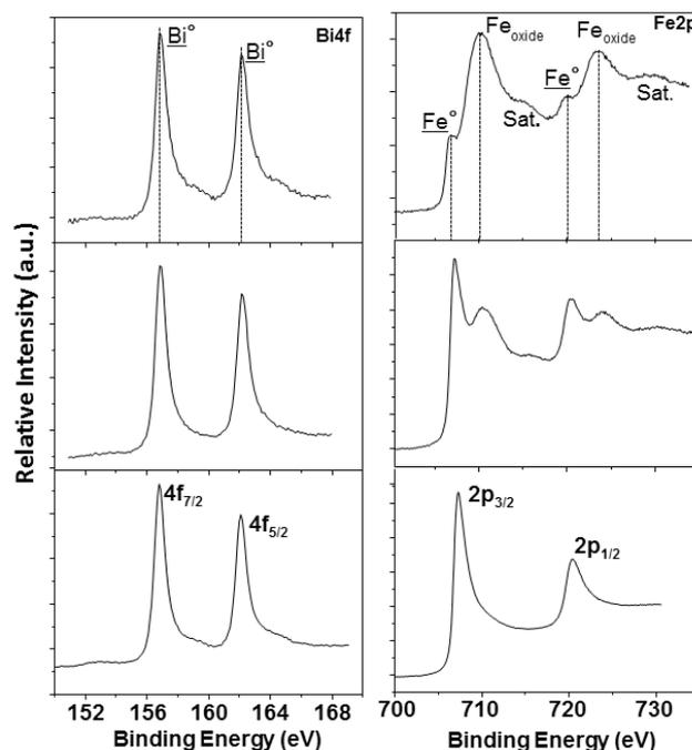
Figure 7: Evolution of the XPS spectra in the Bi-4*f* and Fe-2*p* regions through the different steps of the synthesis. Top: sample *S1* in the presence of amine-borane, middle: sample *S2* after 4h at 110°C under dihydrogen, bottom: sample *S4* after 19h at 150°C under dihydrogen- underlined symbols were chosen for  $\text{Bi}^\circ$  and  $\text{Fe}^\circ$  to include Bi-Fe, respectively Fe-Bi, bonds in the pure metals peaks.
