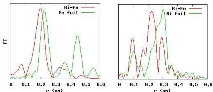
Figure 3: Magnitudes of uncorrected Fourier transforms at Fe  $K$  edge (left) and Bi  $L_3$  edge (right). For easier comparison, the reference foils were adjusted using a scaling factor (0.10 and 0.80 for Fe and Bi, respectively).
