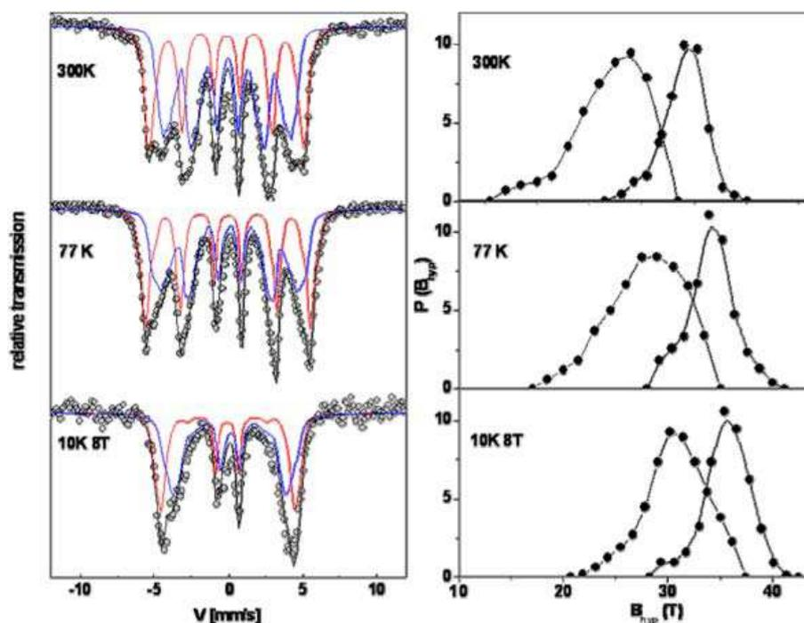
Figure 5:  $^{57}\text{Fe}$  Mössbauer spectra obtained at 300 K, 77 K (without external magnetic field) and 10 K in 8 T magnetic field applied parallel to the  $\gamma$ -beam on powder after 4 months (left side). Spectrum and sub-spectra result from distribution of magnetic sextets based Lorentzian lines which are represented on right side.
