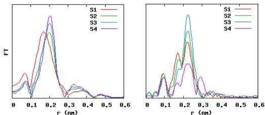
Figure 9: Evolution of the magnitudes of uncorrected Fourier transforms from *S1* to *S4* at Fe *K* edge (left) and Bi *L3* edge (right) - for each edge, all curves are plotted at the same scale.
