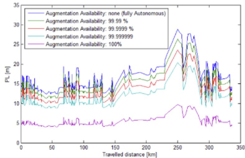
Figure 19: Roma-Pisa railway line. Protection level versus travelled distance with GPS constellation alone. PL is computed without augmentation system in blue (RAIM) and with the support of trackside augmentation systems for the other curves [10].
