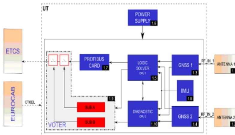
Figure 9: SIL2 architecture of the GRAIL2 project [31].
