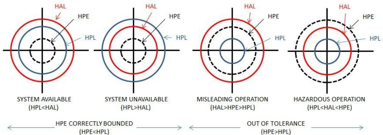
Figure 1: Possible situations obtained with GNSS integrity monitoring
