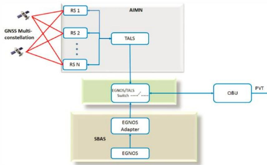
Figure 13: Overview of GNSS LDS System [43].
