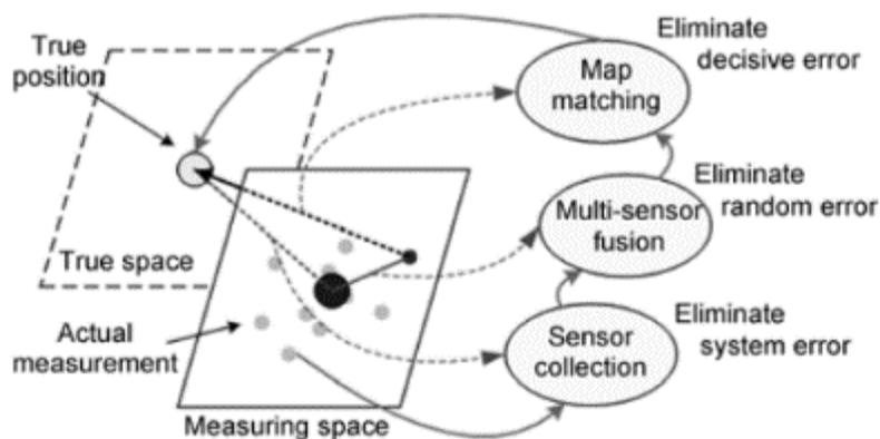
Figure 11: Flowchart of AIMA-aided GNSS-based train integrated positioning [64]
