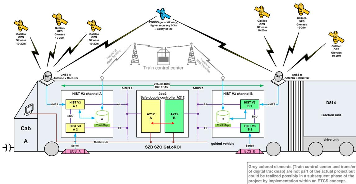
Figure 8: GaLoROI localization unit vehicle equipment [17].
