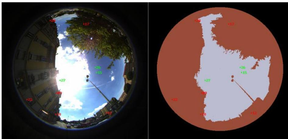
Figure 12: Illustrations of the satellite state detection in a fisheye image on the original image and on classified regions [40].
