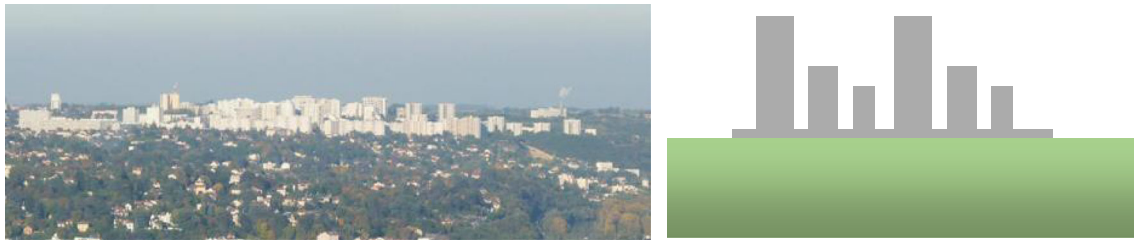
Fig. 6 View of a cluster of buildings ( left ) suggesting the schematic representation of these buildings clamped on a common concrete slab ( right )
