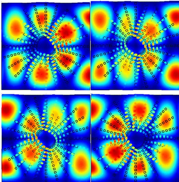
**Fig. 11** Numerical simulation (Comsol Multiphysics) for the proof of concept of the seismic cloak of Fig. 10. Representative snapshots (increasing time steps clockwise from upper left to lower left panel) for a Rayleigh wave coming from the left at frequency 0.5 Hz (color scale with arbitrary unit of energy)
