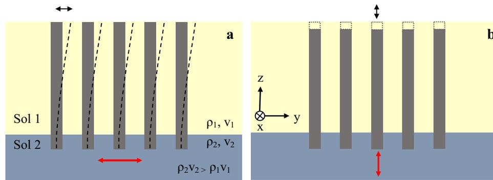
**Fig. 4** Schematic view of principle (*side view*) of vertical columns buried within a soft soil (*soil 1*) and clamped within a bedrock (*soil 2*). These columns undergo bending (**a**) and longitudinal (**b**) motions under earthquake. These local resonances create elastic stop bands at
