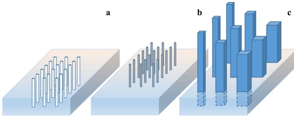
**Fig. 2** From left to right (arbitrary scale): **a** buried columns of deep foundation (piles) or rigid inclusion or holey-ground. **b** Phononic above-ground structure made of vertical metallic elements, inspired from the sculpture of Eusebio Sempere in Madrid. Meseguer and his
